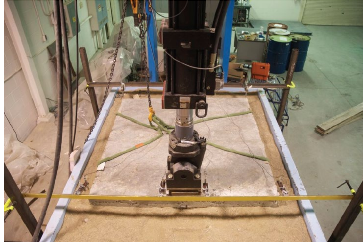
Edge loading: 9cm (FRC) or 15 cm (plain) thickness
