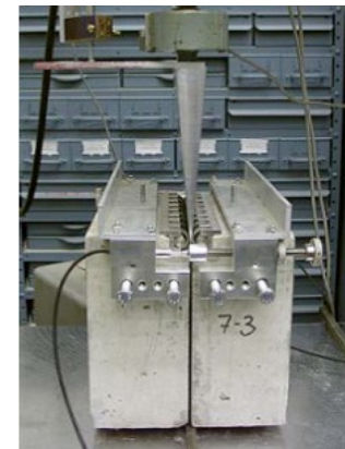
Fig. 2. WST specimen setup
